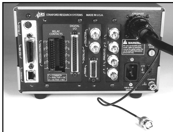
Figure 10-3. The 7-pin plug of the O100C3 cable is connected to the ION GAUGE receptacle on the back of the IGC100. The collector BNC is left unconnected.
